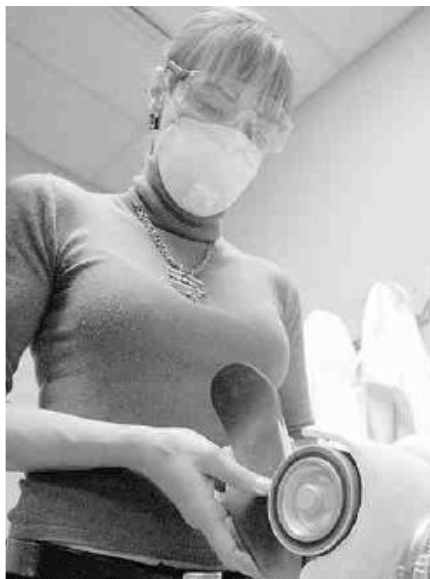
DAVID BEBEE, RECORD STAFF Pedorthist Kim Rau makes a custom adjustment to a foot orthotic with a grinder for specific needs of the patient.
